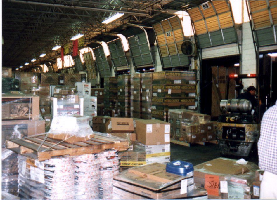
Figure 4: Congestion at a retail crossdock in the northeastern U.S. At the time this photograph was taken, trailers waited an average of 3 days in the yard to be unloaded. This retailer underestimated the difficulting of material handling on the dock.
