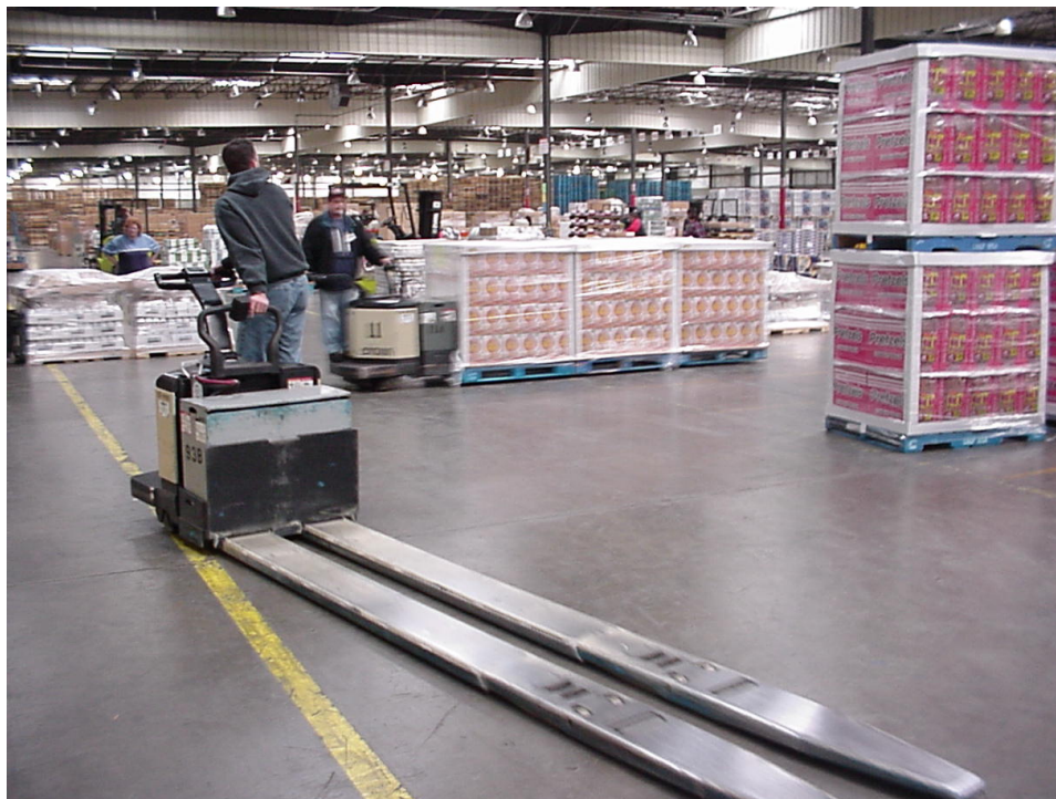
Figure 6: Workers at a Costco crossdock in California. The vehicle closest to the camera can transport 4 pallets at a time. Effective use of this labor-saving device requires vendors to orient pallets consistently in the trailer.
