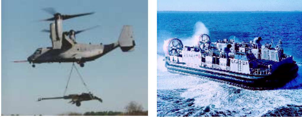
Fig. 1. Transportation platforms for sea based logistics. Left is the MV-22 tilt-rotor aircraft; right is the LCAC air-cushioned watercraft.
