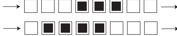
Figure 5: How a staging queue works. Top: Pallets occupy positions 3–5. Bottom: After 2 arrivals and 1 service, positions 4–7 are occupied.
